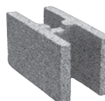
Size: 40×19×20 Max. Weight: 8 kg Strength: 20kg/cm 2 H شکل
